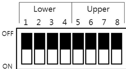
2) Lower bits are set up unit's place and Upper are ten's place.
